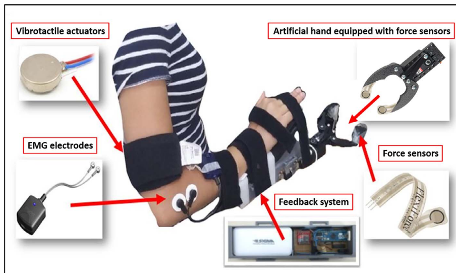
Fig. 1. Myoelectric-controlled hand with vibrotactile feedback system. The signals of the forearm muscles are captured by the EMG Electrodes (lower left), in order to open/close the artificial hand, which has force sensors attached to its inner sides (upper right). When the hand is in contact with an object, the force sensors (lower right) provide vibration to the upper arm via the vibrotactile actuators inside the cuff (upper left). The feedback is operated and controlled through the feedback system (lower middle).
